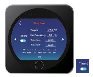
Set your desired parameters by pressing on the <u>Timer 1</u> button and turning it to <u>ON</u>, as shown above.
