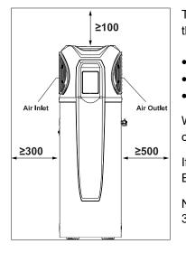
The unit must be installed with sufficient clearances to allow airflow to circulate through the unit, it is advised to keep a **<u>minimum</u>** gap between walls/fences etc of:
