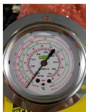
Example of empty (loss of refrigerant)
