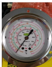
Example of empty (loss of refrigerant)
