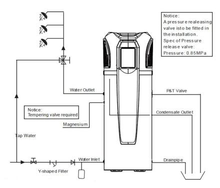
Water Inlet or Outlet Pipes: The specification of the water inlet and outlet thread is BSP3/4 (internal thread). Pipes must be heat-resistant and durable.
