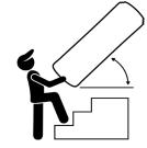
When manually transporting, use the wooden pallet and ropes or straps, ensuring the unit doesn't exceed a 60-degree tilt. After any inclined transport, let the unit rest for an hour before operation.
