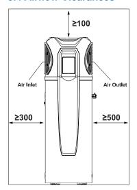
The unit must be installed with sufficient clearances to allow airflow to circulate through the unit, it is advised to keep a **minimum** gap between walls/fences etc of:
