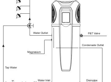
A pressure releasing valve is to be fitted within the installation. Spec of P&T valve: Pressure: 0.85MP Temperature: 99°C
