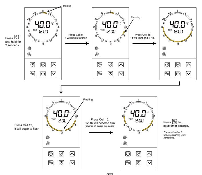
To **cancel** a timer once it has been set, hold down the CLOCK button for 2 seconds until the timer display begins flashing (as you would set the timer).
