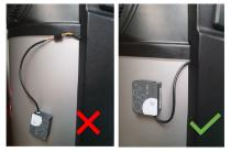
Install the Wi-Fi module upright (cable pointing down), with the connection placed behind the front panel, see left:
