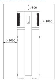
The Evo315-C must be installed with sufficient clearances to allow airflow to circulate through the unit, it is advised to keep a minimum gap between walls/fences etc of:
