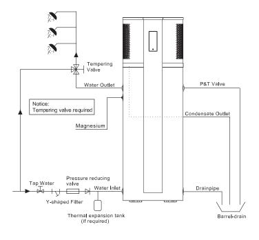
Water Inlet or Outlet Pipes: The specification of the water inlet and outlet thread is BSP3/4 (internal thread). Pipes must be heat-resistant and durable.
