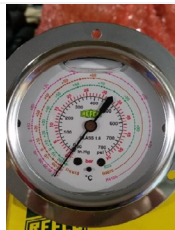
Example of empty (loss of refrigerant)
