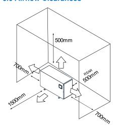
Ensure the heater is installed in a well-ventilated area with plenty of fresh air, a minimum gap between walls/fences, etc., of 700mm on the sides and 500mm at the rear and above the unit. At least 1500mm clearance is required at the front.
