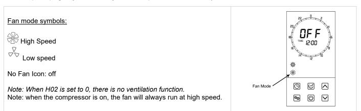
When the parameter HO2 is set to 1, press the for 2s.
