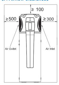
The Evo150-1 must be installed with sufficient clearances to allow airflow to circulate through the unit, it is advised to keep a minimum gap between walls/fences etc of:
