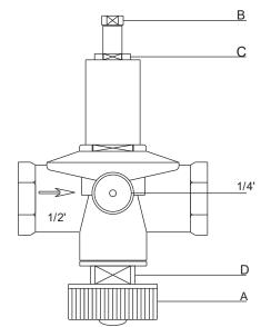
NOTE: There are two connections for the water pressure meter in the central section of automatic filled-water, where the water pressure meter can be connected directly and display the set pressure. The screw cap ( C ) must be tweaked after adjusting the filled-water pressure.
