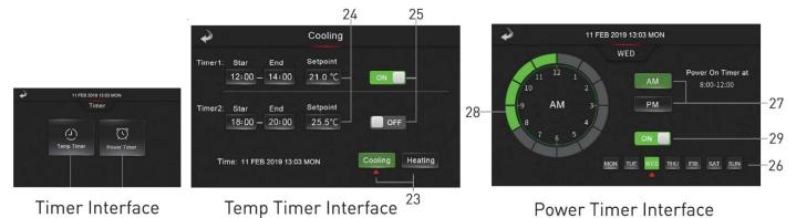
After pressing the 'Timer button from the main interface, select from Temp Timer or Power Timer.
