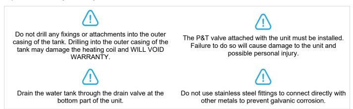
Note: A pressure releasing valve is to be fitted within the installation. Spec of P&T valve: Pressure: 0.85MP Temperature: 99°C
