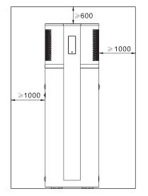
The Evo315-C must be installed with sufficient clearances to allow airflow to circulate through the unit, it is advised to keep a minimum gap between walls/fences etc of:
