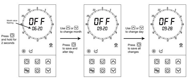
Note: Format is mm/dd Example: The unit will start up on September the 28<sup>th</sup>.
