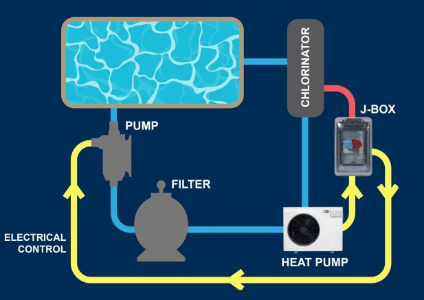
Note: Make sure you allow power requirements for the water pump that is on the same circuit as the heat pump.
