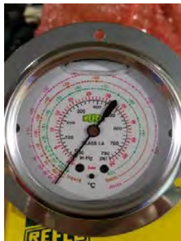
Example of empty (loss of refrigerant)
