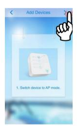
Then select the > arrow in the right screen and select switch device to AP mode (See below)
