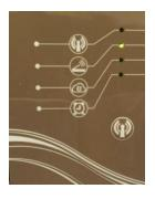
On your Wi-Fi module, the second light down should now be yellow and within a few seconds the third light will start flashing to show communication with the internet.
